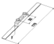
16 101.6201 Height: 8.0 mm Hole distance: 32.0 mm For shaft height: 35.5 mm
