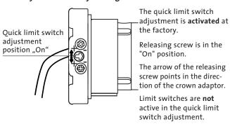
**Note:** The maximum limit switch range is 35 revolutions of the shaft.
