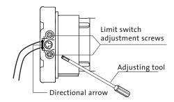
Turn the adjusting tool of the DOWN limit switch adjustment screw in the + or - direction until the final end position is reached.
