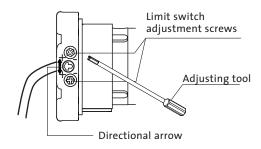
4. Turn the adjusting tool of the UP limit switch adjustment screw in the + or – direction until the end position is reached. One turn of the limit switch adjustment screw represents approx. 60° of turning of the winding shaft.
