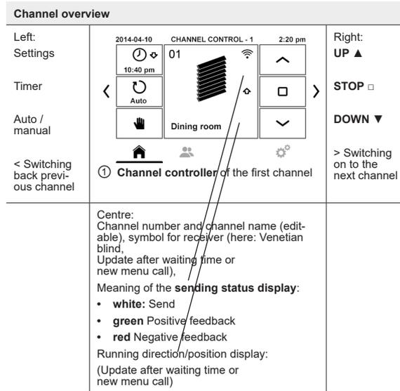
Fig. 3 Channel control channel 1
