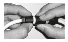
Place the union nut on the contact carrier and tighten with a torque of 1.5 Nm.
