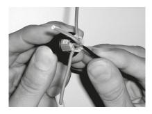
3. Clip the wire (0.34–0.75 mm²) into the colour coded wire guides
